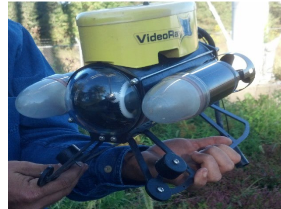
Early in 2024, all water tanks were inspected. (Submersible ROV shown above)
